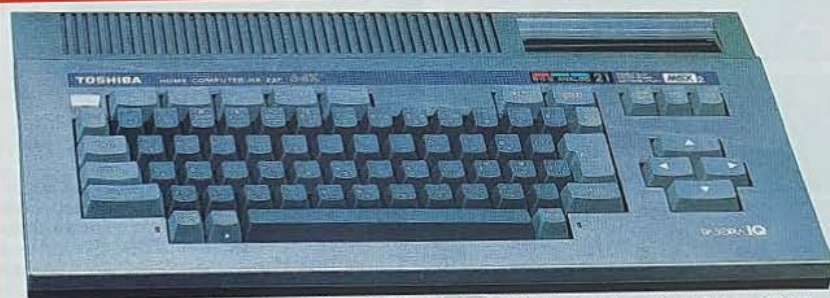
Toshiba, Pasopia, IQ, HX-23F, MSX II, CPU : Z80A, ROM : 48 KB (MSX 2 - Basic) + 48 KB, RAM : 128 KB, VRAM 128 KB, VDP : 9938
